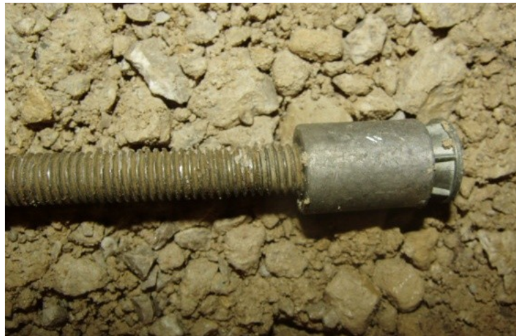
Figure 3.9. An Example \frac{1}{2} - 13 Ready Rod and Korker
